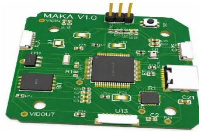
Figure 4 3D PCB model of the STM32 F405-based flight controller (dimensions: 4 × 4 cm)
